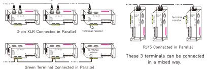
$5.3\ {\ The\ connection\ diagram\ of\ AMP\ signal\ amplifier\ terminal:}$
