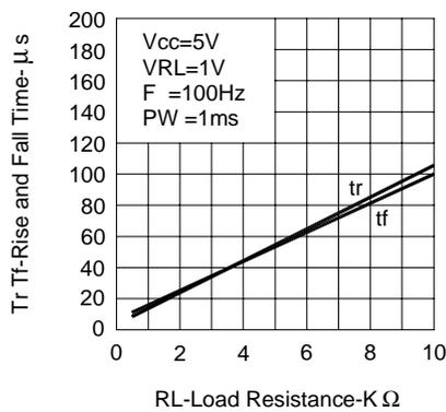
FIG.3 RISE AND FALL TIME VS LOAD RESISTANCE
