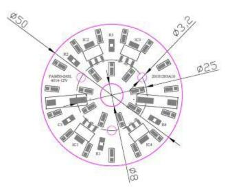
Notes: Use in conjunction with constant Voltage LED drivers 12vdc 10W min Ensure thermal management to maintain LED junction temp Tc Max 85°C Higher intensity versions are available on request Specifications may be subject to change without notice
