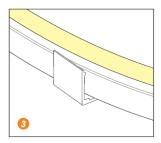
Put the light emitting surface upwards, then insert the LED strip into the fixed
