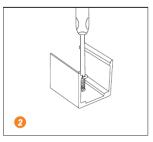
Adjust the fixed clips to the appropriate place, use a screwdriver to fix the screw.
