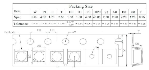
2.1x2.1mm, White LEDs Surface Mount PLCC-4 White LEDs
