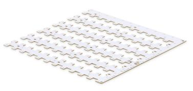
The Fortimo LED Square 5000 lm (380 x 380 mm) design leads to cost effective lighting solutions while generating 5000 lm. A system consists of one LED Square module and driver. The luminaire design can have a smaller exit window than the traditional 600 x 600 mm design, or differentiate on light distribution in combination with designed optics.
